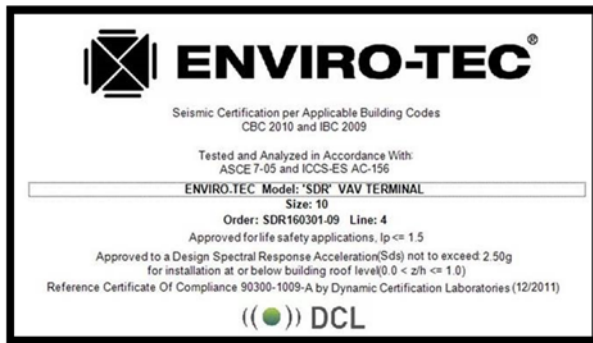
FIGURE 1 – SAMPLE LABEL FROM A SEISMIC RATED VAV TERMINAL UNIT
